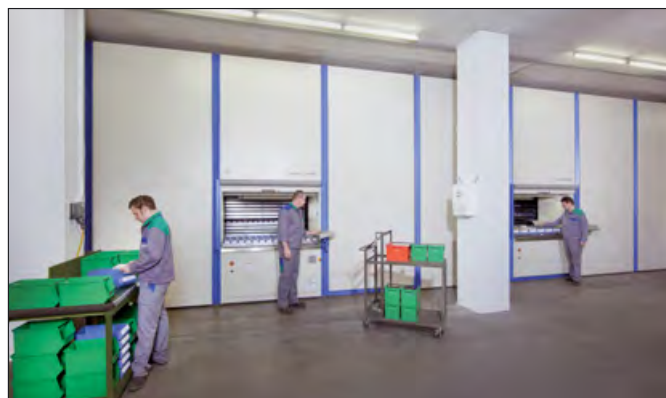
Two Hänel Multi-Space® units, each almost 393.10" wide, constitute the central store for the production hall
