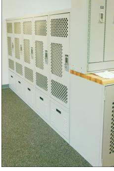
provide secure storage for personal items while still promoting optimal ventilation. Directly below each locker door, the planning team opted for louvered drawers fitted with drying racks, which allow agents to follow best practices for storing body armor. DigiLock technology allows agents to open lockers with a PIN code, and a master badge allows designated supervisors to open any locker in the room.
