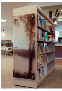
3Form sheets with custom imagery onto the laminate end panels was done to ensure that they were clearly visible, instead of viewing metal shelving through the translucent material.
